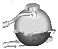
Check to see if coolant is visible in the coolant surge tank. If the coolant inside the coolant surge tank is boiling, do not do anything else until it cools down. See *Engine Overheating* ⇒ 249.
