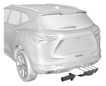
To remove the hitch cover, if equipped:
