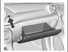
To open, press the button. Close the glove box manually.
