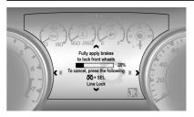
6. Press the brake pedal firmly to move the bar graph to 100%.
