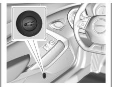
From inside the vehicle, press  $\iff$  on the lower portion of the driver door.
