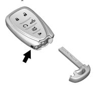
Press the button on the side of the remote key and pull the key out. Never pull the key out without pressing the button.
